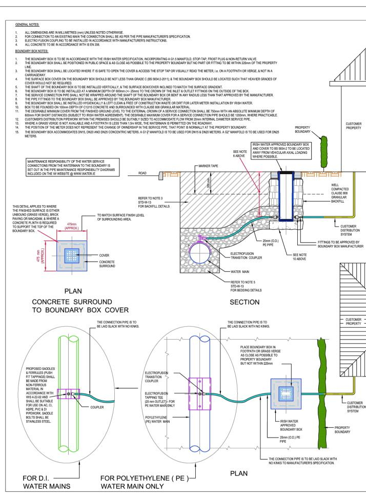
STD-W-03 CUSTOMER CONNECTION AND BOUNDARY BOX (25mm OD PIPE)
